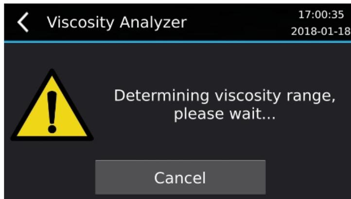
6. The platform will move down to a starting position 2 mm above the vat film in the material. It will then move down 0.1 mm and wait until the material settles, recording the distance above the vat film and the time it takes to settle. It will repeat this until the settle time is above the settling time threshold and then interpolate the distance above the vat film which corresponds to the settling time threshold. The distance is then displayed as the viscosity range.
