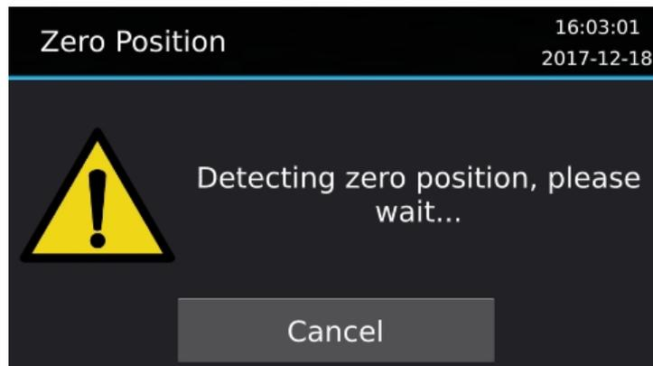
16. Pressing Cancel will stop the “detect zero position” process and skip to the “Home vertical axis?” screen.
