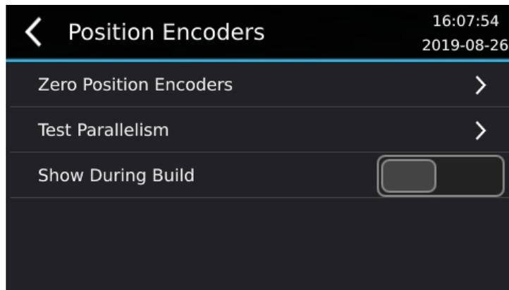
2. Activating the option “Show During Build” will show the position encoders values and blue dot while building similar to the Zero Position Encoders screen.
