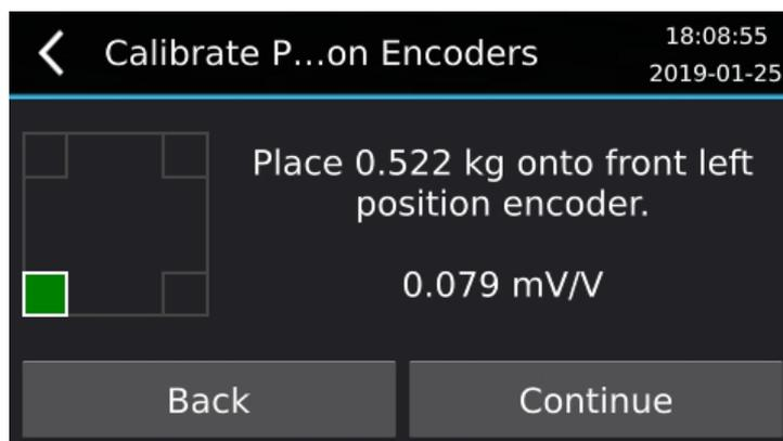
If the mV/V value has not increased enough, it will stay flashing white and pressing Continue will change the indicator to solid red to indicate the calibration for the position encoder has failed. Press Continue.
