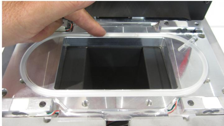
12. If all of the position encoders were successfully calibrated, all indicators will be green and you can proceed to reattach basin and tighten the 4 black screws which hold the basin in place. Do not insert the build tray. Press "Finish".
