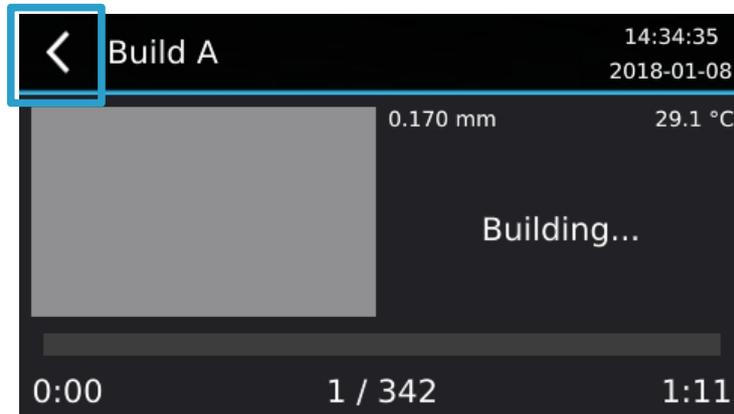
When the build is paused you can raise or lower the build using the screen buttons. You can continue the build with the Resume button or abort the build with the Cancel button.
