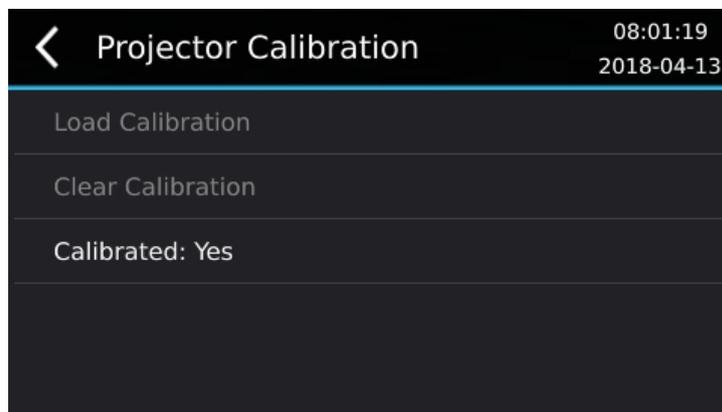
“Load Calibration” loads the calibration from a replacement projector onto your system. This will only be enabled if there is calibration data available to load from the projector.
