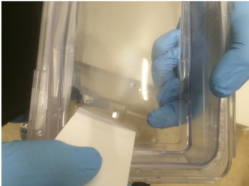
3. Place a finger on the underside of the vat film at a corner of the cured rectangle. Your finger will provide support for the next step.
