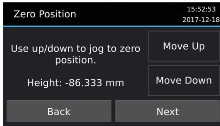
8. Use the “Move Up” and “Move Down” buttons to lower the build platform to the lowest position.
