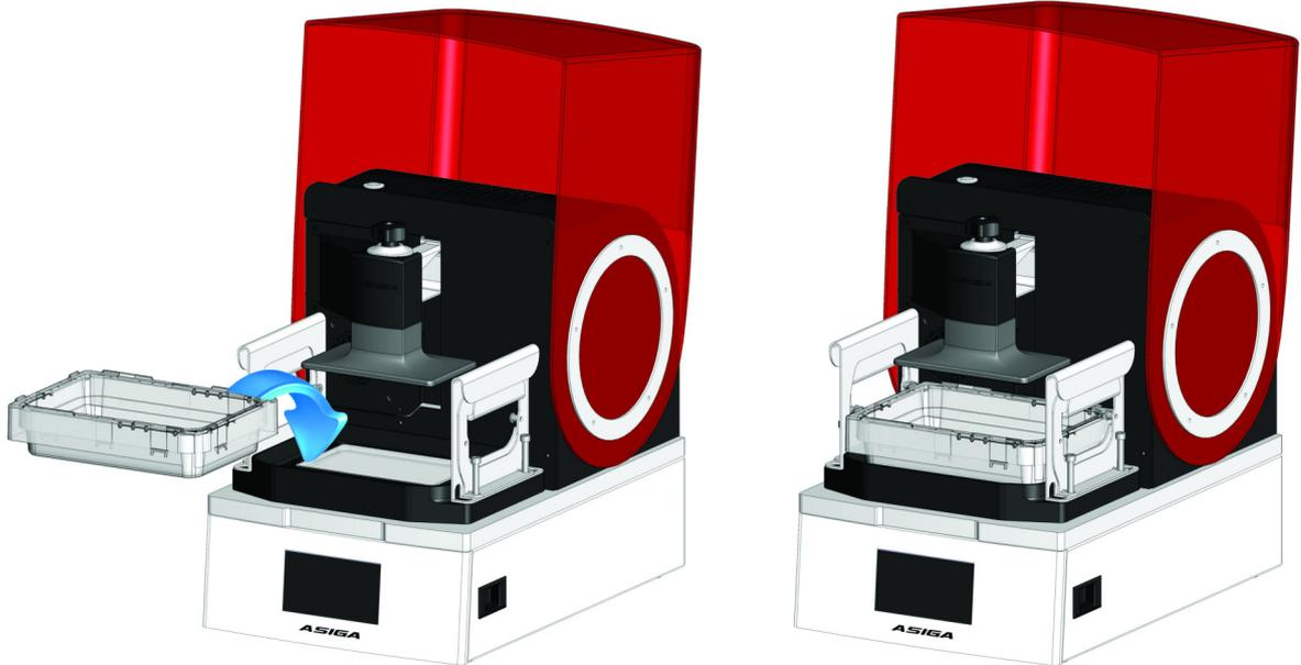
3. Grip the handles and pull up and tilt inwards until the teeth grip over the edge of the vat.
