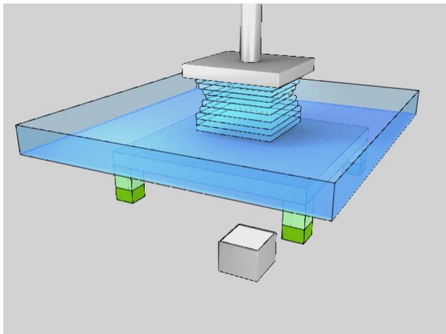
4. A cross-sectional image of the object being constructed is projected onto the underside of the vat film, causing photopolymer to harden in the shape of the image.
