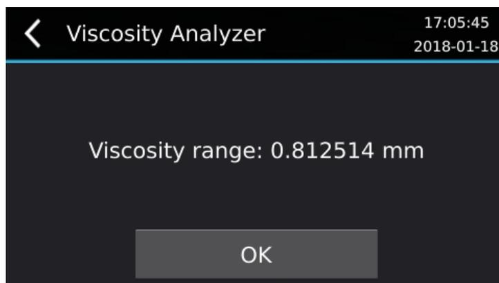
The data recorded that is used to determine the viscosity range is logged to "Debug Information" which may be accessed through the "System Information" tab of the web interface.
