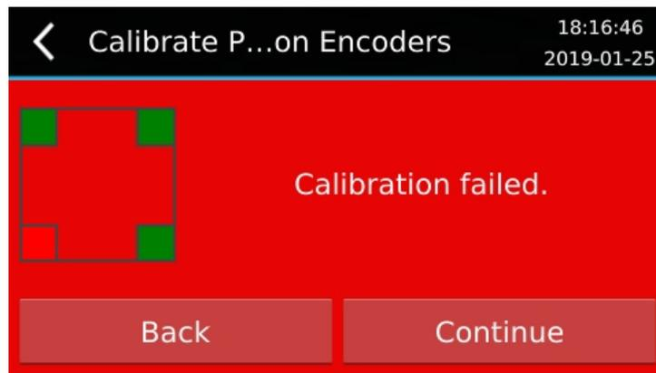
Press Back to go back to the previous screen or press the back arrow to go back to the menu. You may press Continue but the machine will not function correctly. After pressing Continue, reattach basin and tighten the 4 black screws which hold the basin in place. Do not insert the build tray. Press "Finish".
