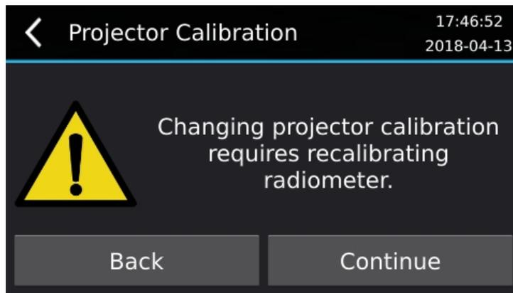
This means that after you load calibration or clear calibration, you will need to recalibrate the internal radiometer – please refer to Calibrate Radiometer in CHAPTER 8. Press “Continue” to proceed.
