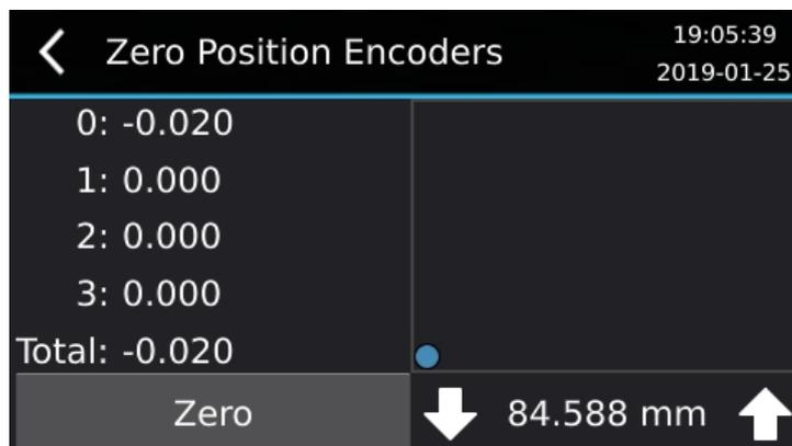
3. The empty square region shows a two-dimensional deflection map of the build envelope with a blue dot at the zero center. Pressing the up and down arrows will move the vertical axis up and down. The current height in mm above the zero position is shown between the arrows.
