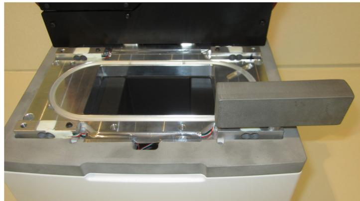
Once the calibration weight has been placed on the position encoder, the indicator should change to solid green.
