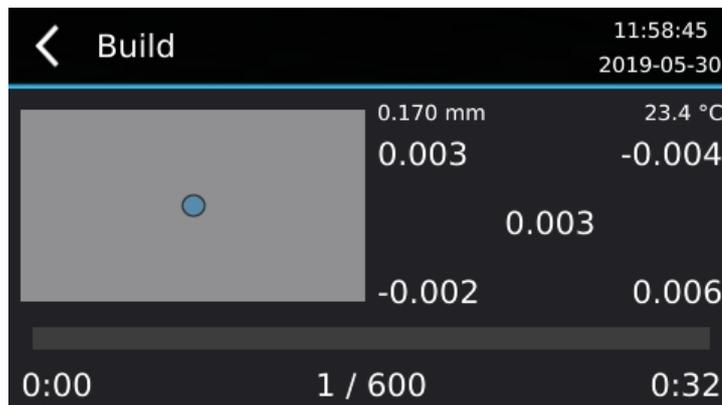
Deactivating the option “Show During Build” will show the text “Building...” while building instead of the position encoder values and blue dot.
