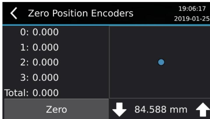
6. The process is complete. The blue dot should be in the center of the square.
