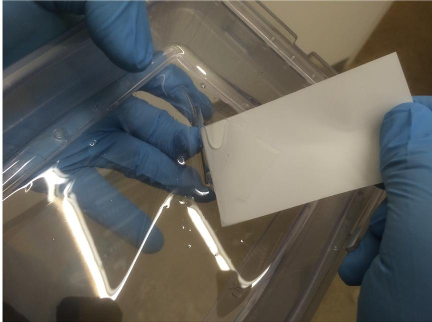
5. Remove the cured rectangle in one piece and dispose of it.
