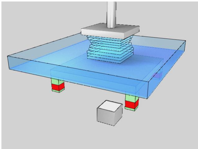
3. Four position encoders at each corner of the glass plate precisely monitor the mechanical deflection between the glass plate and the model under construction. The process monitors the deflection until it is relieved.
