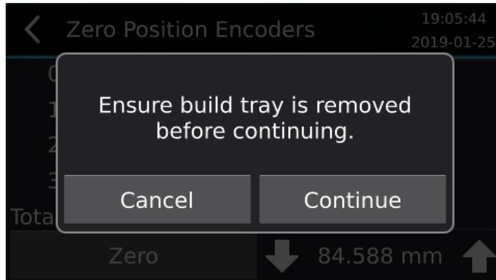
5. Remove the build tray from the machine. **There should be no objects in the build tray area or anything pressing on the machine.** The machine should be on a level surface in a low vibration area. Press “Cancel” to abort the process, otherwise, when ready, click “Continue” to record the zero position.
