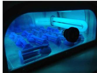
The parts may still be tacky on the surface due to atmospheric oxygen inhibiting the photo-curing reaction. Full surface cure can be obtained by immersing the parts in a liquid to displace the oxygen and irradiating the immersed parts. Suitable liquids include oil, water and glycerol.
