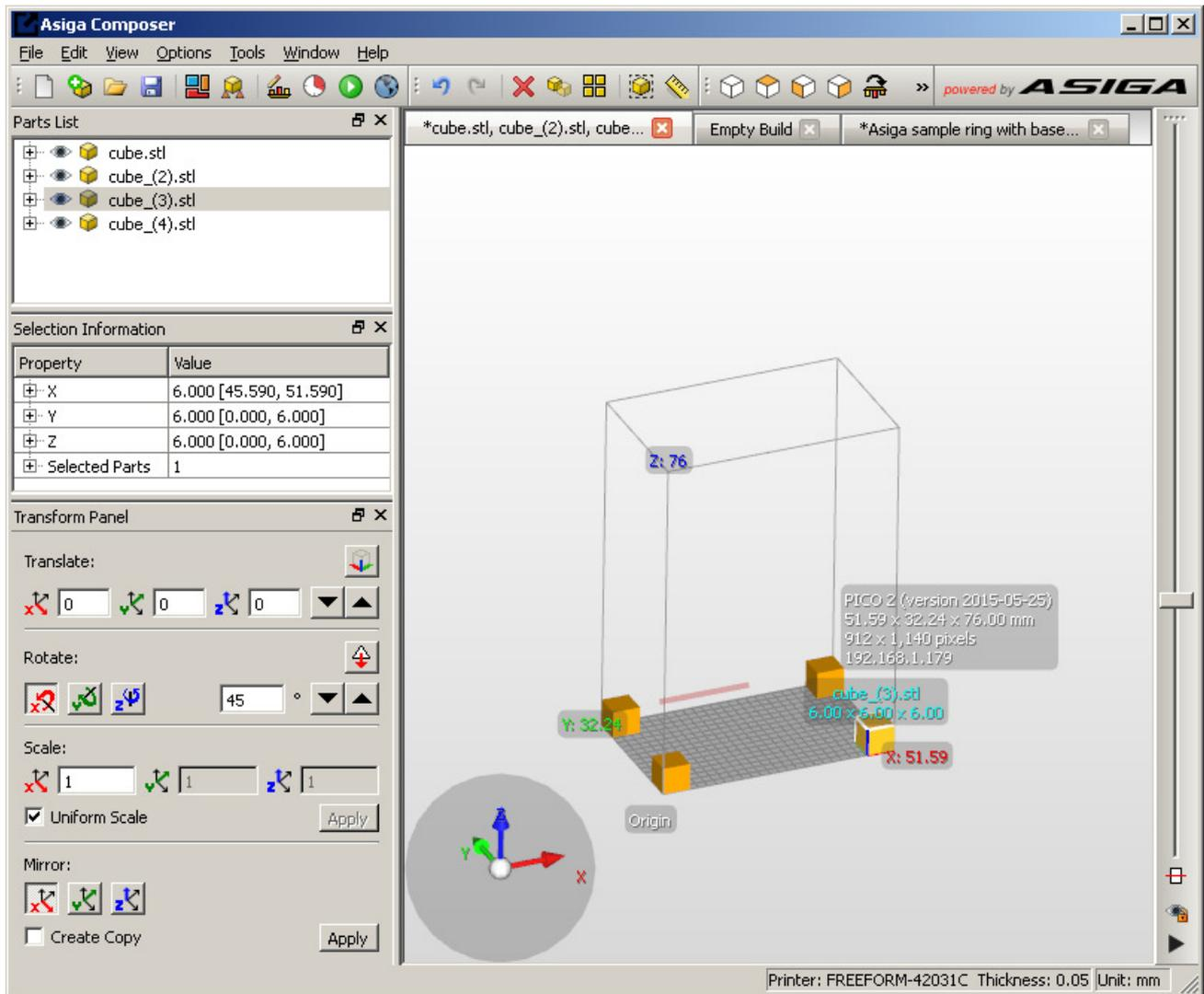
The measured X and Y span values are entered into the appropriate fields and the “Save” button is clicked to save the changes.
