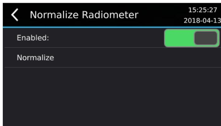
The Enabled toggle controls whether to use previously recorded normalization readings to improve the radiometer response across the image area. This does not need to be changed at all. It will be automatically enabled after performing the radiometer normalization process either automatically after Calibrate Radiometer is completed or manually normalizing by clicking Normalize.
