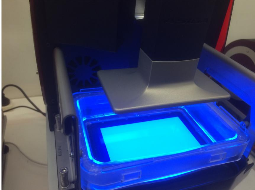
2. Remove the vat from the machine. There will be a cured rectangle of material adhered to the vat bottom.
