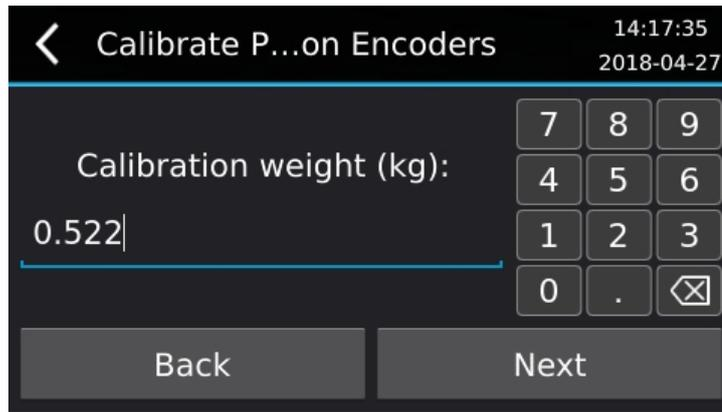
7. Place the calibration weight onto the front left position encoder (the calibration weight should only be touching the position encoder and not any other part of the machine). A square indicator is shown on the display for each position encoder. The indicator for the current position encoder will flash white.
