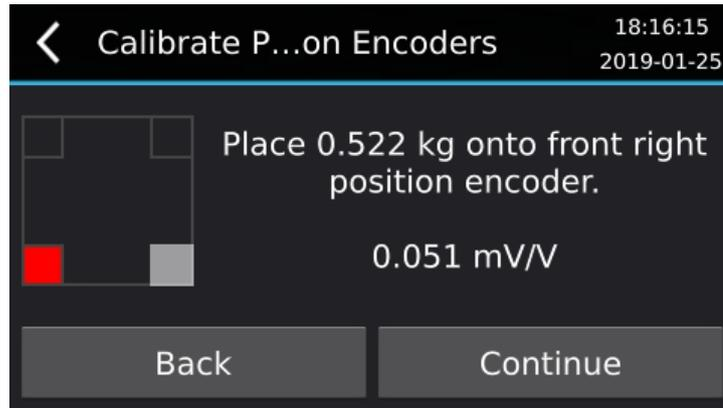
8. Place the calibration weight onto the front right position encoder (the calibration weight should only be touching the position encoder and not any other part of the machine).
