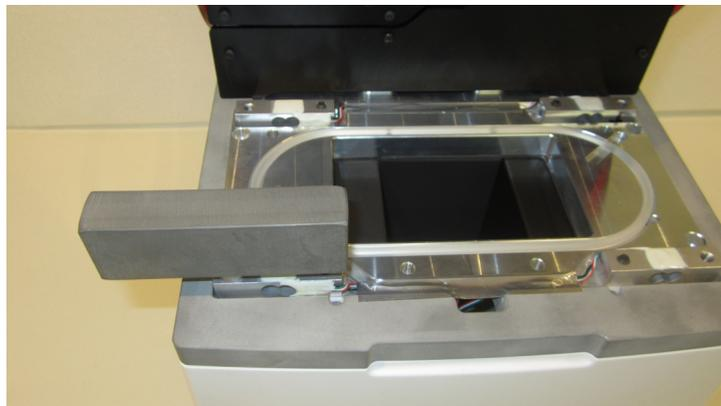
Once the calibration weight has been placed on the position encoder, the indicator should change to solid green.
