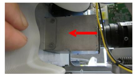
9. Rotate the lens with your fingers to adjust the focus.
