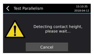
The platform will move down and the contact height will be detected when it comes into contact with the dome nut.
