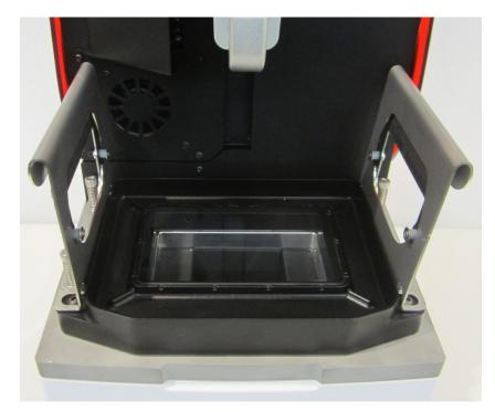
3. Remove the 4 black screws which hold the basin in place.
