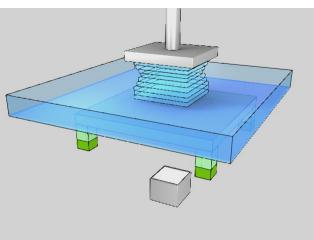
4. A cross-sectional image of the object being constructed is projected onto the underside of the vat film, causing photopolymer to harden in the shape of the image.
