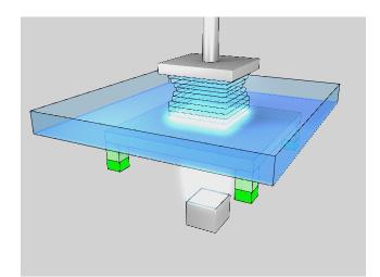
5. The model is lifted out of the vat to separate it from the vat film.
