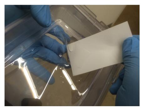
5. Remove the cured rectangle in one piece and dispose of it.
