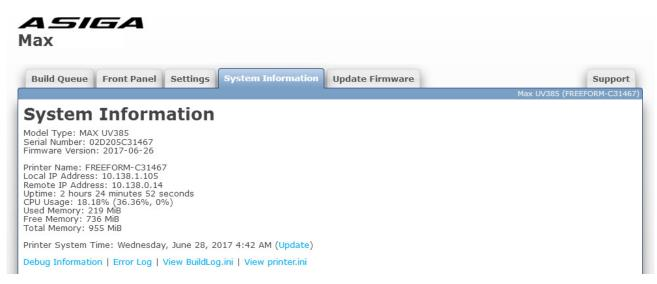
Model Type – This will be "MAX" for a MAX printer
