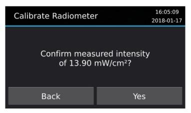
6. The internal radiometer will automatically be normalized to improve the radiometer response across the image area by illuminating different areas and measuring the change in radiometer readings. This will take less than 8 seconds to complete.
