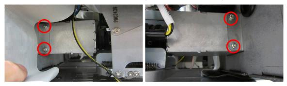
8. Slide the dust protection chamber towards the front of the machine to access the lens.
