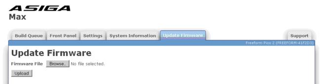
Firmware files have the file extension ".fw". You can click Browse to select a firmware file and then click Upload to upload it. The printer will verify the firmware is valid and if it is, it will be added to the list of firmware in the System > Firmware Version menu on the front panel. You can then select the desired firmware from the Firmware Version menu to update to the selected version. The printer will keep the 5 most recently uploaded firmware files.
