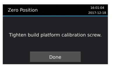
14. Detect the zero position. The feedback from the position encoders may be used to automatically detect the zero position of the build platform. To run the automatic detection process, click "Yes".
