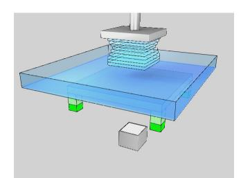
2. The model is moved downwards to one layer-thickness above the bottom of the vat. The movement squeezes photopolymer resin out from the gap between the model and the Teflon film. Viscous forces oppose the motion, resulting in mechanical deflection of the apparatus.
