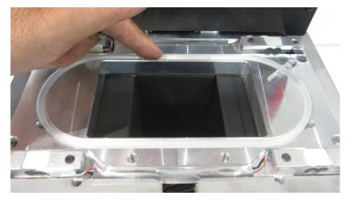
12. If all of the position encoders were successfully calibrated, all indicators will be green and you can proceed to reattach basin and tighten the 4 black screws which hold the basin in place. Do not insert the build tray. Press "Finish".
