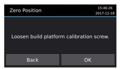
4. Loosen the build platform calibration screw. This can be done with a 4mm hex key hand tool which is included in the MAX Calibration Tool Kit. When the screw is properly loosened, the build platform should be able to move freely up and down and rotate around the horizontal axes of the machine.
