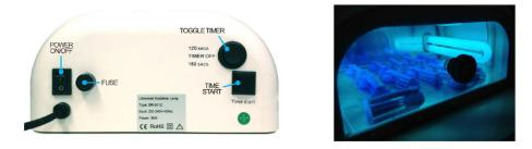
The parts may still be tacky on the surface due to atmospheric oxygen inhibiting the photocuring reaction. Full surface cure can be obtained by immersing the parts in a liquid to displace the oxygen and irradiating the immersed parts. Suitable liquids include oil, water and glycerol.
