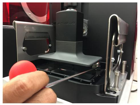
6. Move the dome nut to the front left corner. The dome nut should be resting within the glass and completely underneath the platform.
