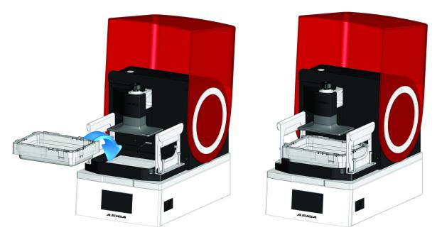
3. Grip the handles and pull up and tilt inwards until the teeth grip over the edge of the vat.
