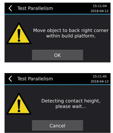
The platform will move down and the contact height will be detected when it comes into contact with the dome nut.
